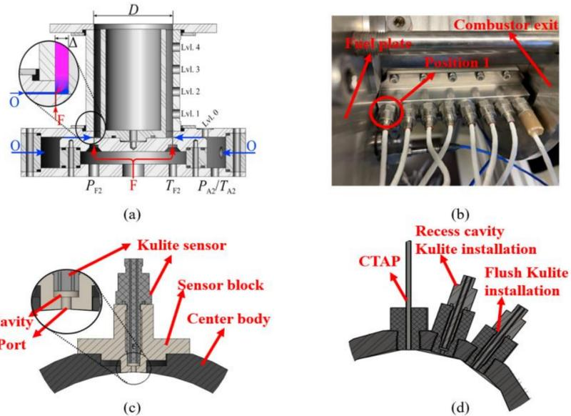
(a) TU Berlin's RDC, (b) recessed sensor block on the RDC, (c) cross section of a recessed mounted Kulite sensor, and (d) Kulite sensors in flush, recessed and CTAP configuration.
